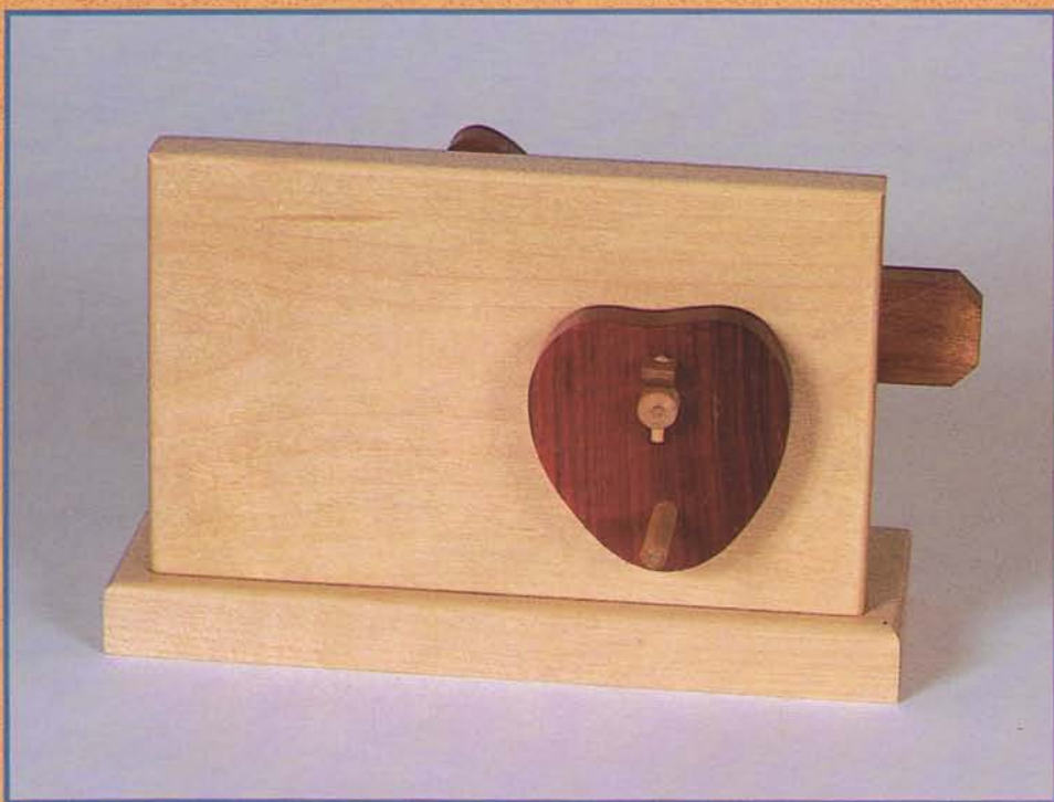
The Positive-Action Cam provides absolute control of the position of its follower, under all conditions of operation. Top: a front view of the Positive Action Cam. Above: a rear view.
